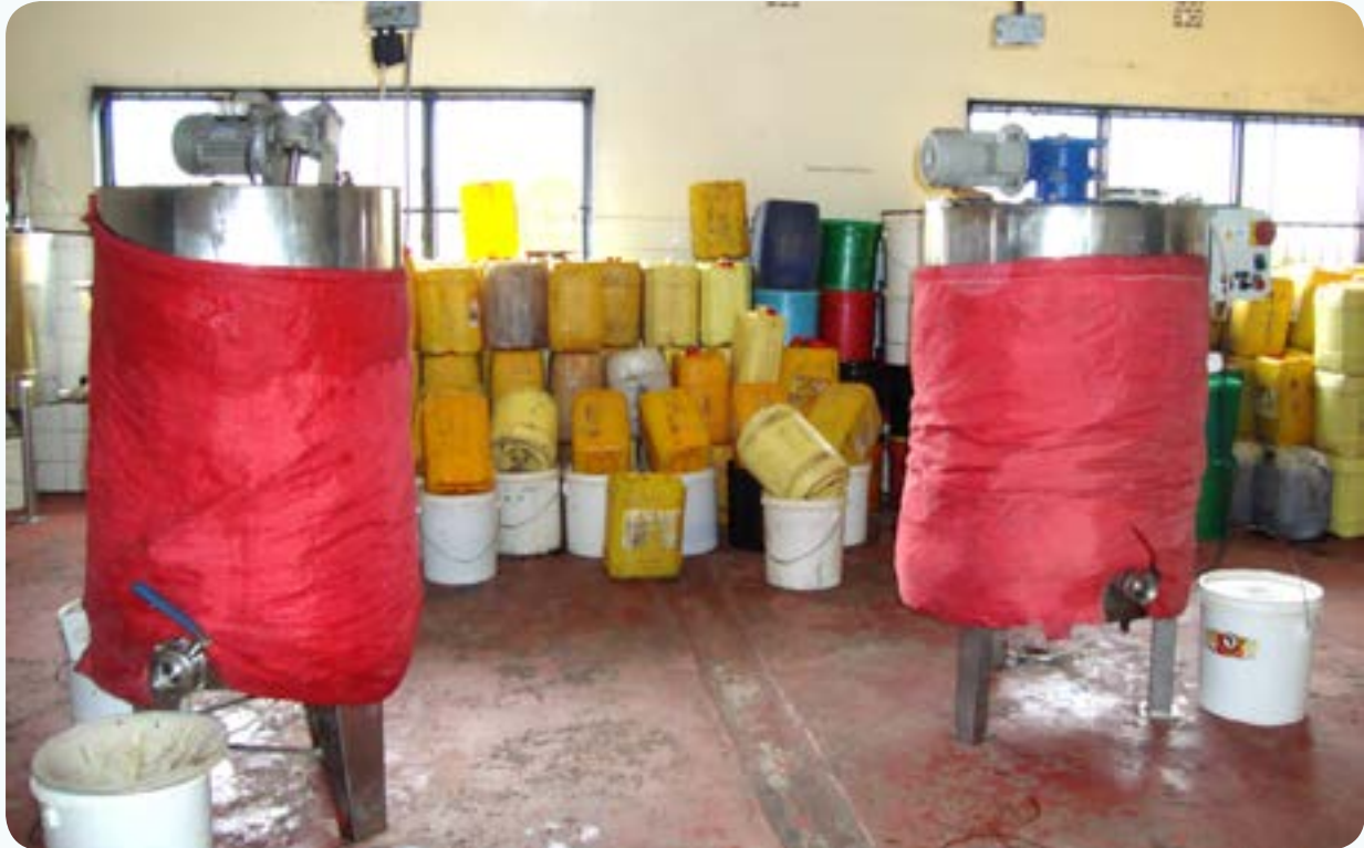
At headquarters, the honey is pasteurized to help separate particles. It is then sieved and stored in buckets until cool.
